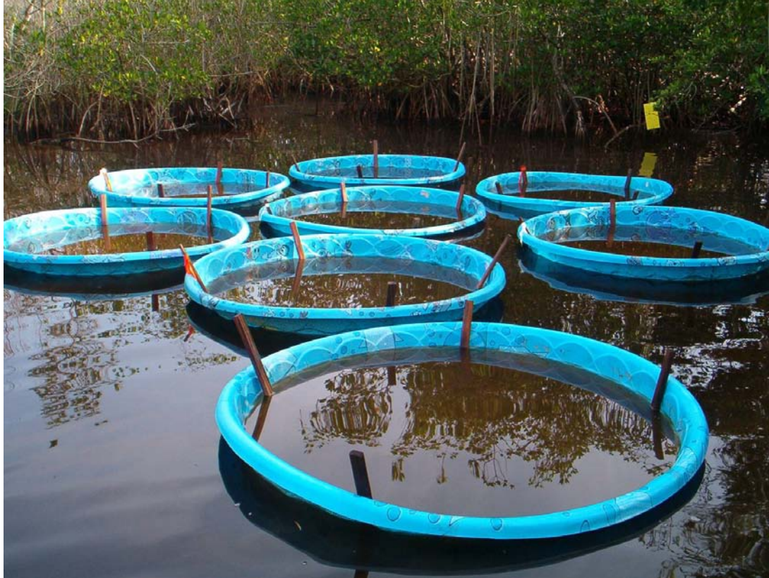
Figure 2. "Natural pools" were established with each plastic ring anchored by 4 wooden stakes driven in at an angle to prevent movement due to tidal influx. Before Agnique ® MMF application, the pools were checked to make sure the plastic rings stay in contact with the sediment soil in a brackish marsh impoundment, Vero Beach, FL.
