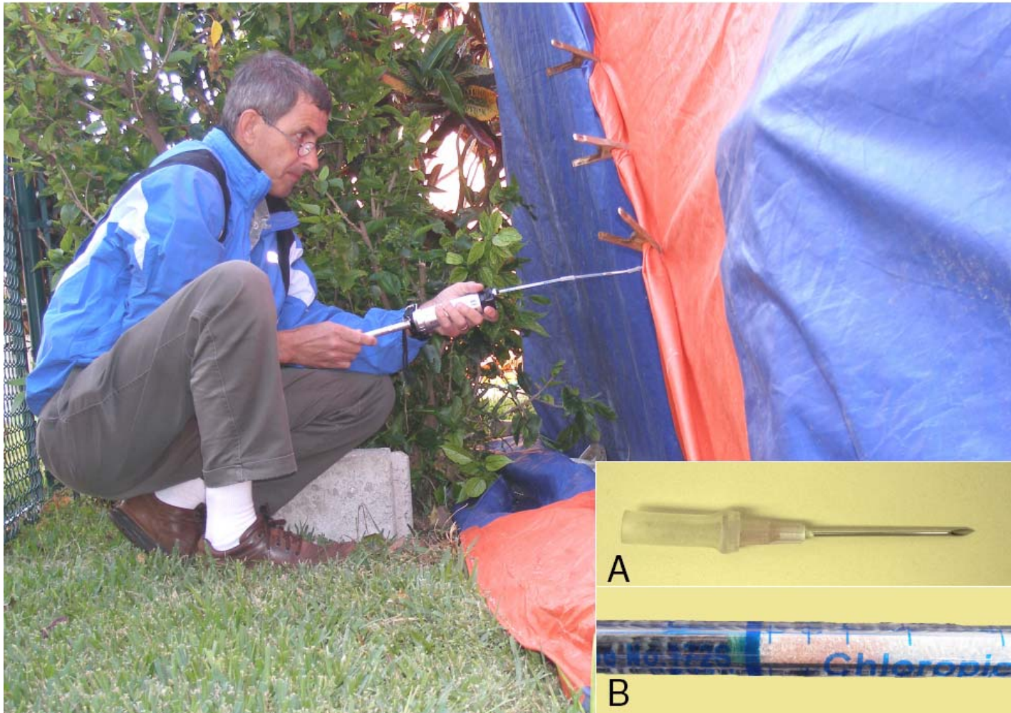
Figure 1. Chloropicrin was measured through the tarpaulin seal of a fumigated structure using a 14-gauge hypodermic needle (A) connected by rubber sleeve to the “pretreat” tube. Another sleeve was used to connect the pretreat tube to the measuring tube (B) which was attached to the pump apparatus.
