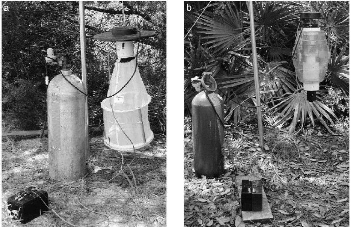
Fig. 2. (a) American Biophysics Corporation (ABC) surveillance light trap. (b) MM-X control trap.
